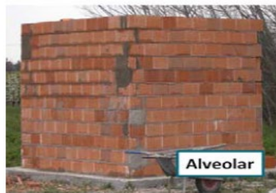
Figure 7 The alveolar brick TES test structure at Lleida University in Spain (Farre, 2016)
