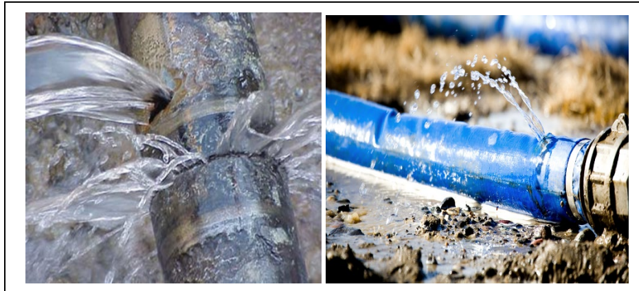
Figure 3: Illegal connection and leaking pipes
