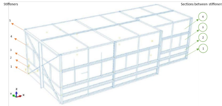
Figure 7. Model of the rectangular tank on ABAQUS (Wajtaszak, 1936).
