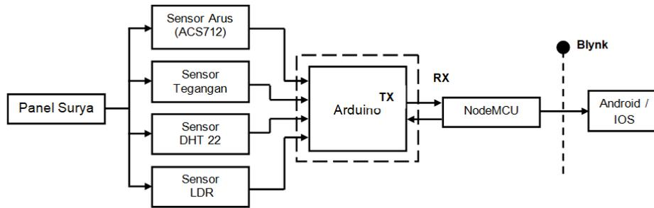
Figure 1. Block diagram of the solar panel performance monitoring system
