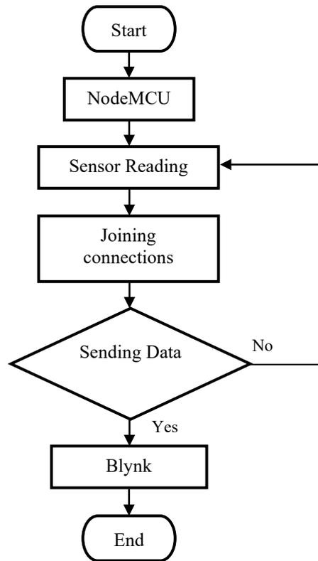
Figure 4. The flow diagram of the nodeMCU program
