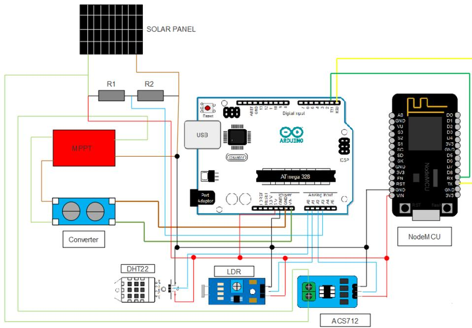
Figure 2. Monitoring circuit design of the performance of solar panels.
