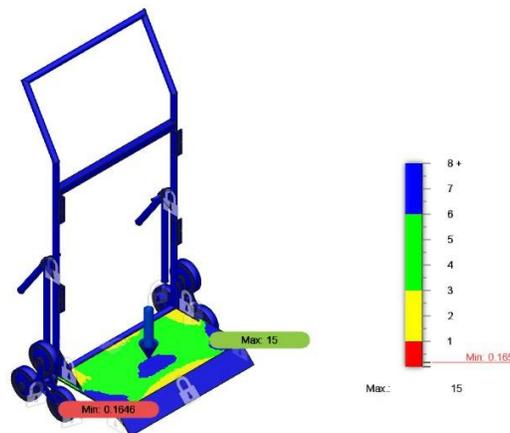
Fig. 1. Final Trolley Simulation using Autodesk Fusion 360
