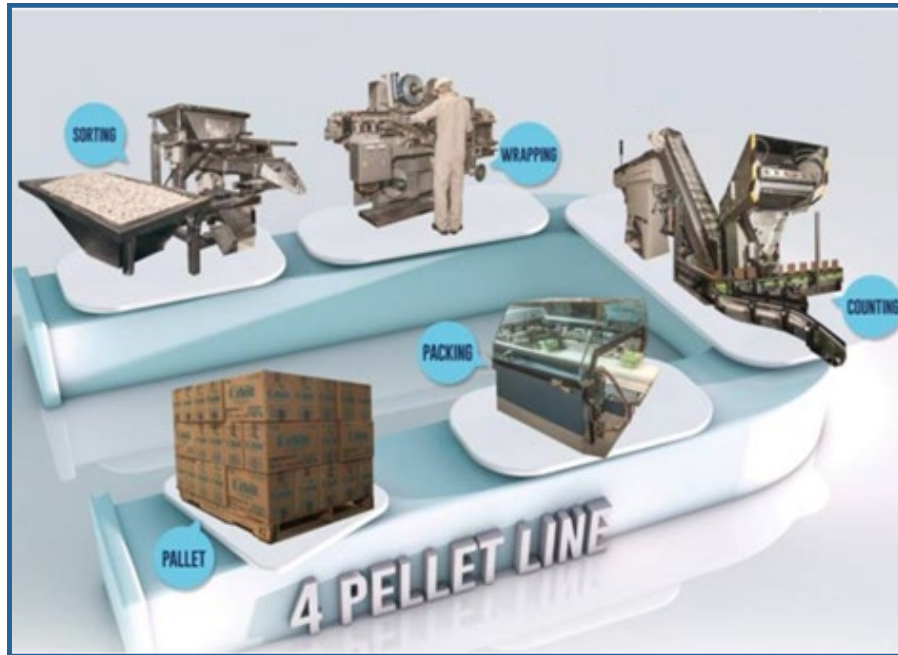
Figure 1. Chewing gum process flow
