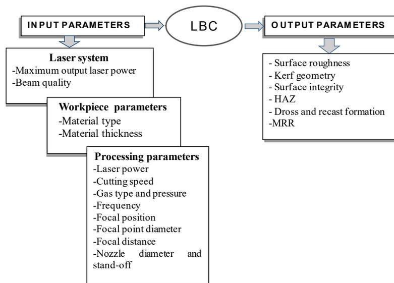
Figure 3. Laser beam cutting process parameters
