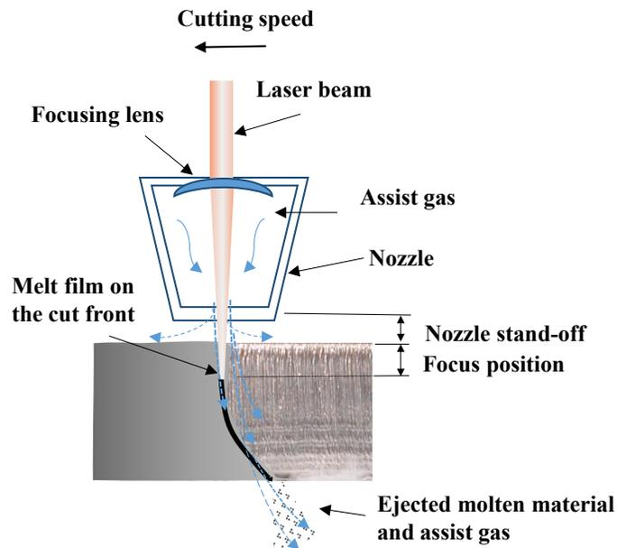
Figure 2. Schematic representation of laser beam fusion cutting
