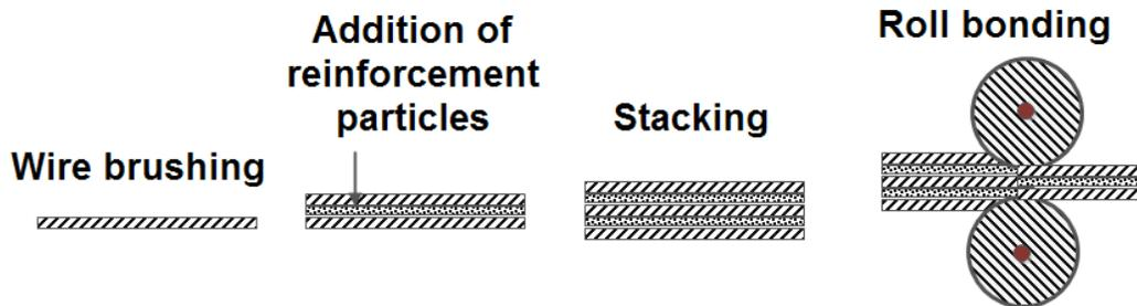
**Figure 4** Schematic representation of accumulative roll bonding process
