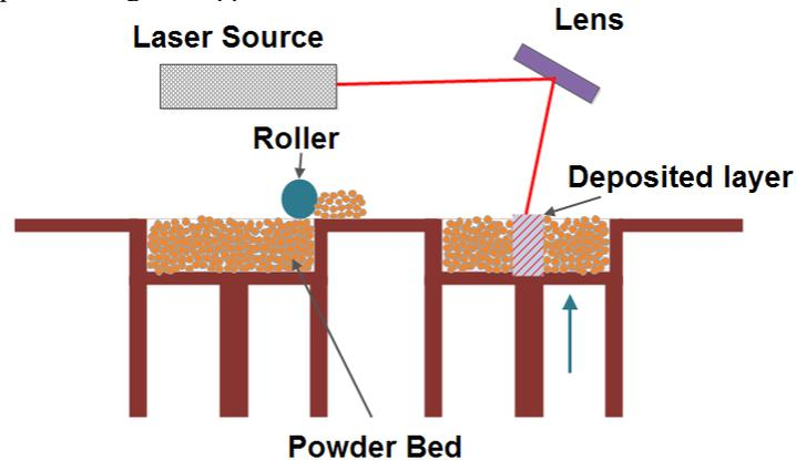
**Figure2** Schematic representation of powder-bed additive manufacturing
