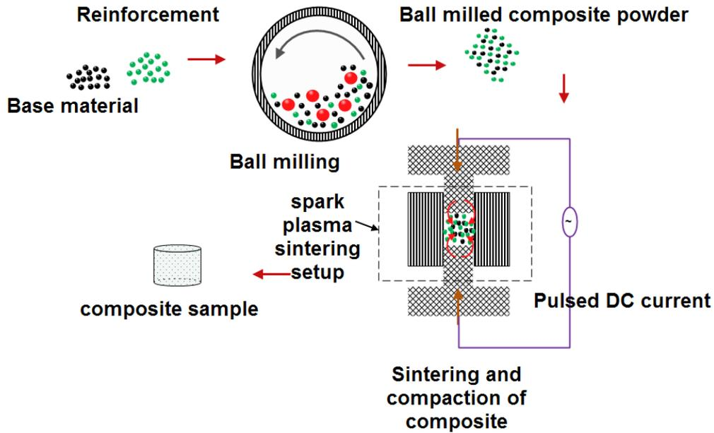
Figure 3 Schematic representation of spark plasma assisted sintering
