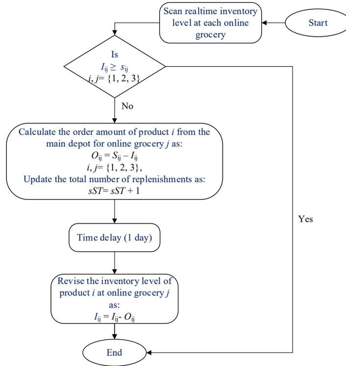
Figure 4. Flowchart of continuous inventory control in simulated model.
