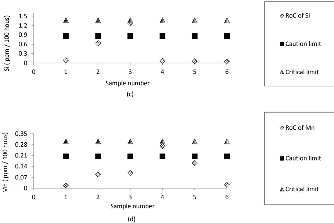
Figure 1. Rate of change steel alloy components (a) Iron, (b) Vanadium, (c) Silicon, (d) Manganese
