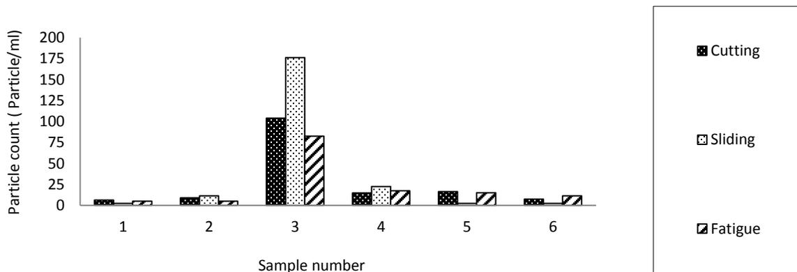
Figure 2, Distribution of wear modes in the gearbox
