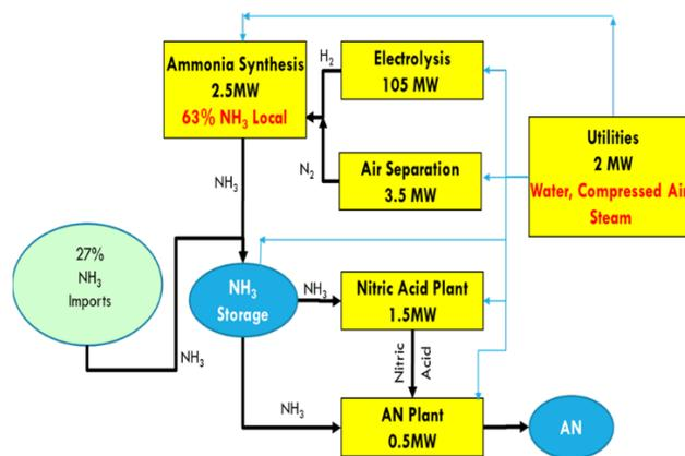
Figure 1: Installed plant configuration
