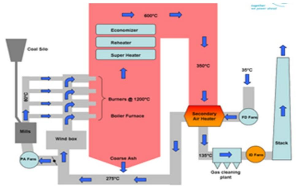
Figure 1: Overview of Process – Coal & Gas Cycle.
