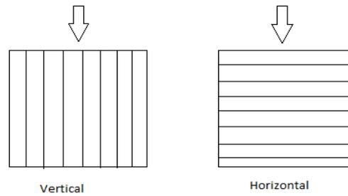
Figure 1: A visual representation of the Load applied vs Material printed axis.
