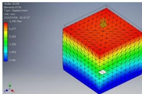
Figure 2: load of 25Mpa applied to the y-axis.
