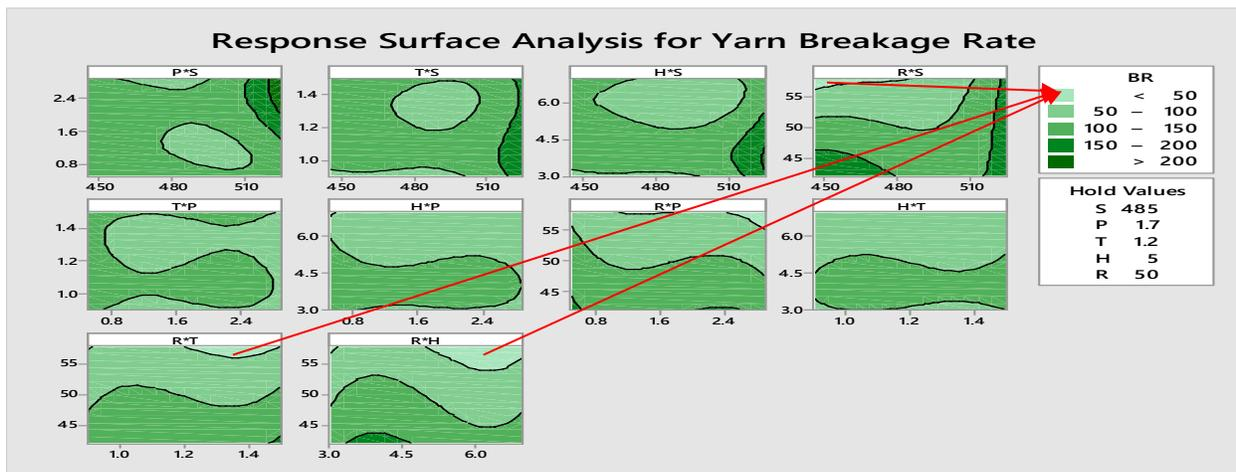
Figure 4: Possible Regions for Optimal Parameter Values of Looming Process, the Pale Green Region that is Represented by the Line Depicts Smallest Yarn Breakage Rate
