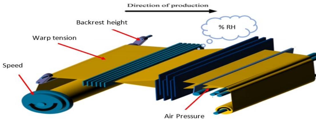
Figure 2: Schematic diagram of looming system that elaborates selected, but machine related, parameters indicated by arrows (Source: F. Cloppenburg, Y-S Gloy and T. Gries (2015))
