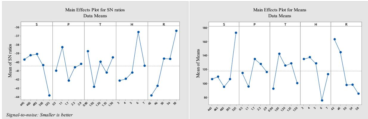
Figure 3: Plot of S/N ratio for yarn breakage, the high pick points depict the high signal value that are capable to dominate the noises
