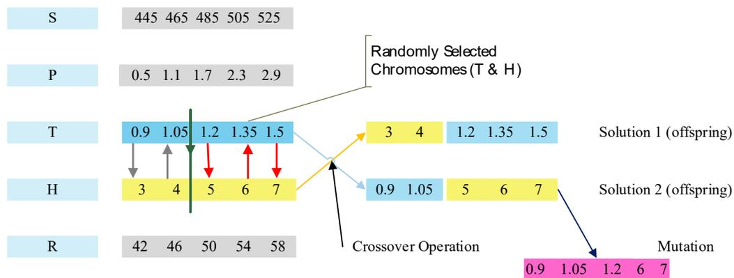
Figure 5: Working Principle of GA Optimization, Each Offspring Signifies the Possible Solutions
