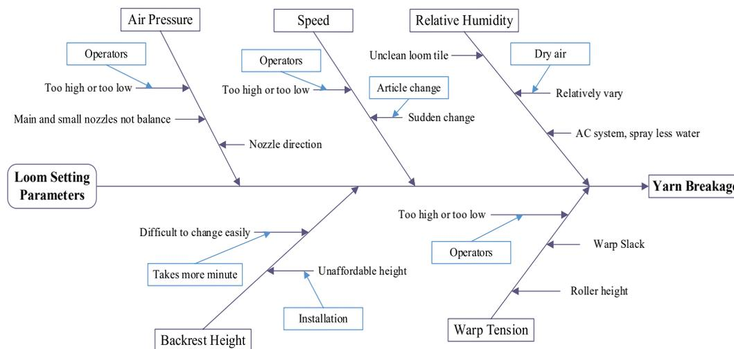
Figure 1: Cause and Effect Analysis of loom process parameter for yarn breakage
