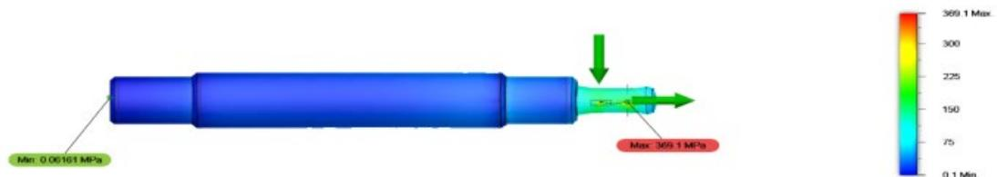
Figure 3: Centrifugal Pump Shaft at varying stress distribution from 100 MPa during operation
