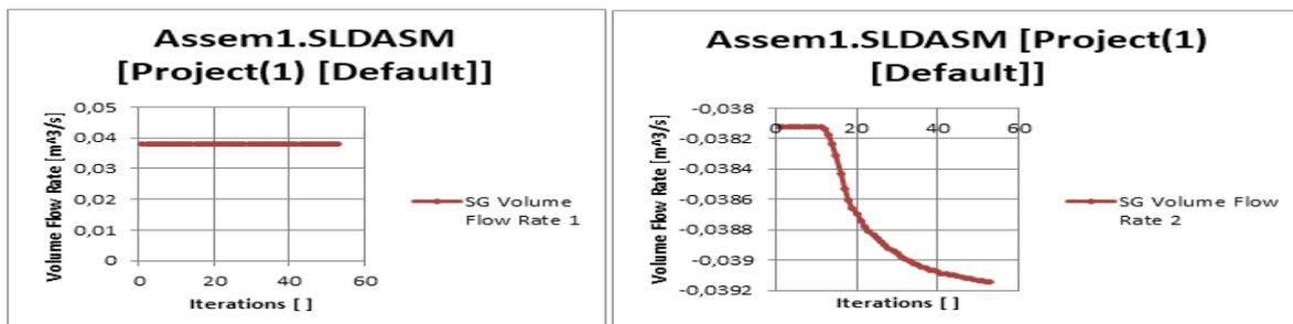
Figure 4: Volume flow rate both at inlet and exit of the tunnel
