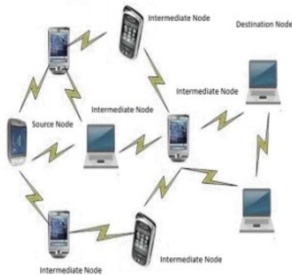
Figure 2. Typical Architecture Diagram for Mobile Ad-hoc Network (MANET)
