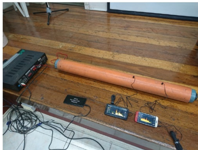
Figure 2. Impedance tube setup
