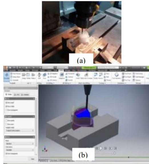
Figure 4. Molds Actual Fabrication and CNC Simulation
