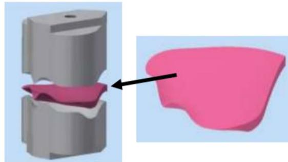
Figure 2. Conceptualized Upper and Lower Molds and Rose Petals
