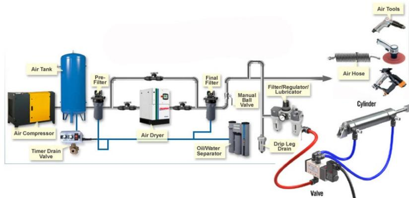
Figure 1. Pneumatic System Components
