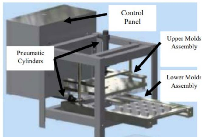
Figure 3. Molding Machine (3D CAD Model) Isometric View
