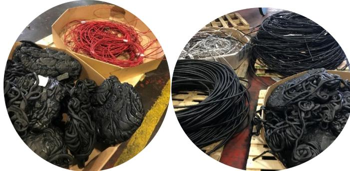
**Fig 1. Plastic coating/sheathing defects**
