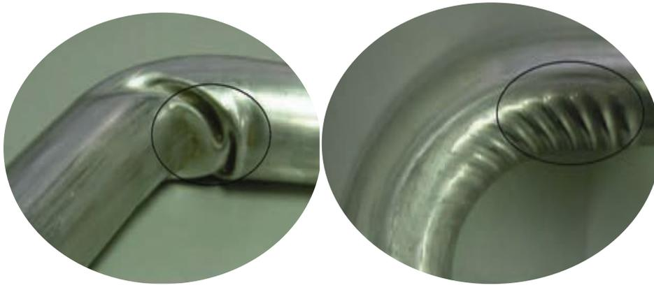
**Fig 3. Tool defects in Pipe bending**
