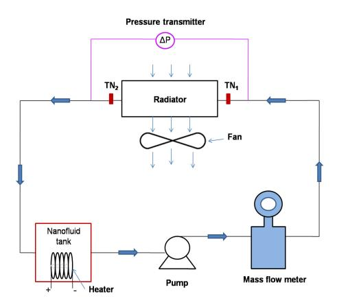
Figure 1.0 Schematic view of Experimental setup
