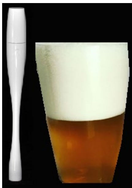
Figure 2. Ultrasound equipment to generate foam
