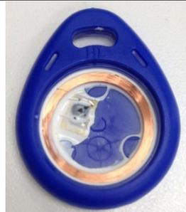
Figure 3. TAG with damage encapsulation
