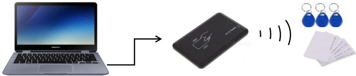
Figure 1. Portable RFID system integrated by a computer, a reader and TAG
