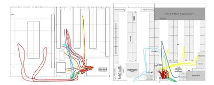
Figure 2. Spaghetti diagram for movements of a typical warehouse worker (before and after improvements)
