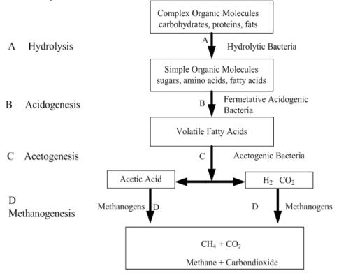
Figure 1. Anaerobic Digestion Process
