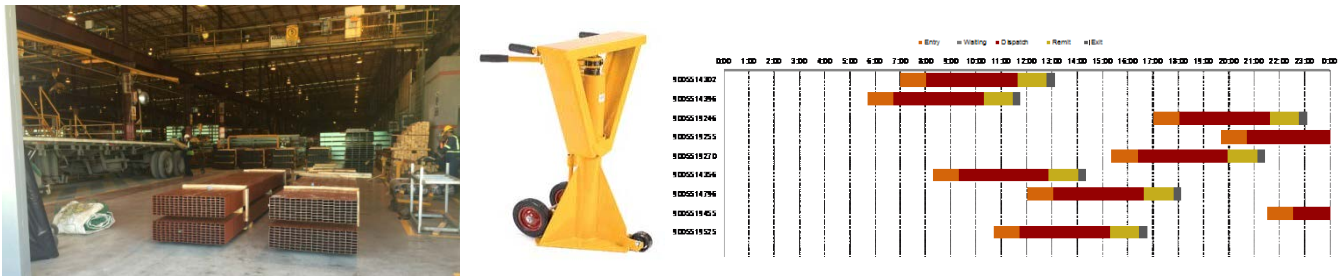
Figure 4 Preparing Material in Advance for Transportation, Device for Enabling Drop & Pick & Scheduling Truck Loading
