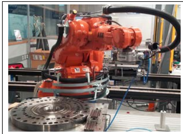
Figure 1. The robotic setup with force torque control
