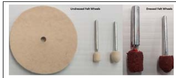
Figure 4. Undressed and Dressed Felt Wheels.
