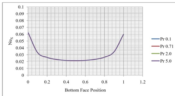
Figure 15. Distribution of Local Nusselt Number at Bottom face at different Prandtl Number
