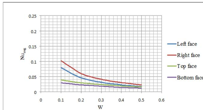
Figure 26. Variation of Average Nusselt Number at different faces with Slender Body Width
