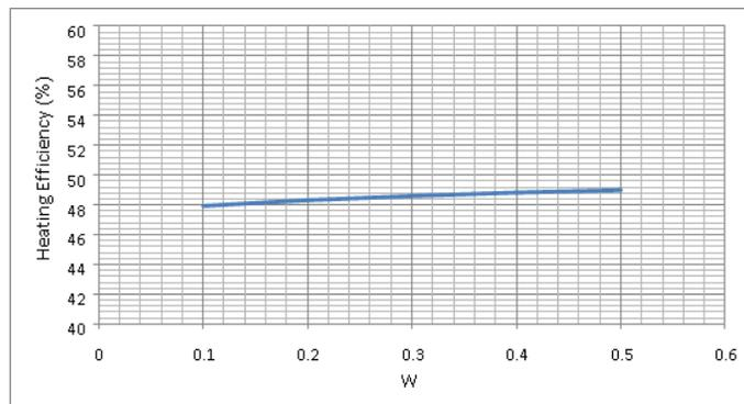
Figure 28. Variation of Efficiency With Slender Body Width
