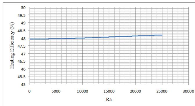
Figure 11. Variation of Efficiency with Rayleigh Number
