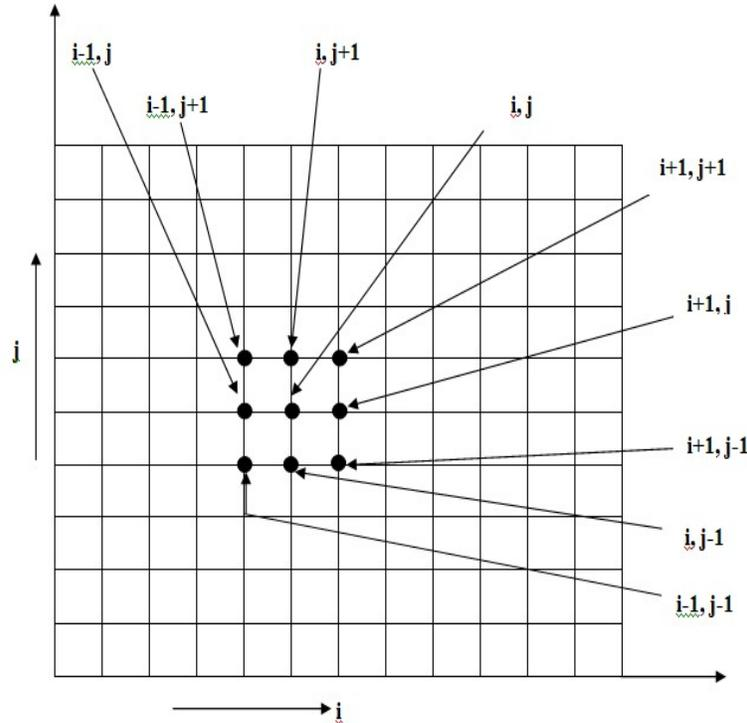
Figure 1. Grid and Co-ordinate system in the Computational Domain
