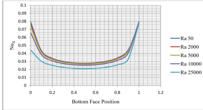
Figure 5. Distribution of Local Nusselt Number at Bottom face at different Rayleigh Number
