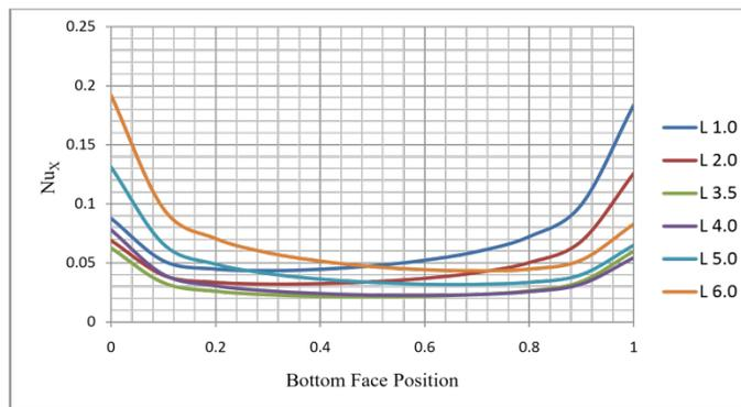
Figure 22. Distribution of Local Nusselt Number at Bottom face at different Locations
