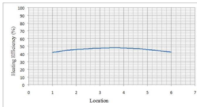
Figure 25. Variation of Efficiency with Slender Body Locations
