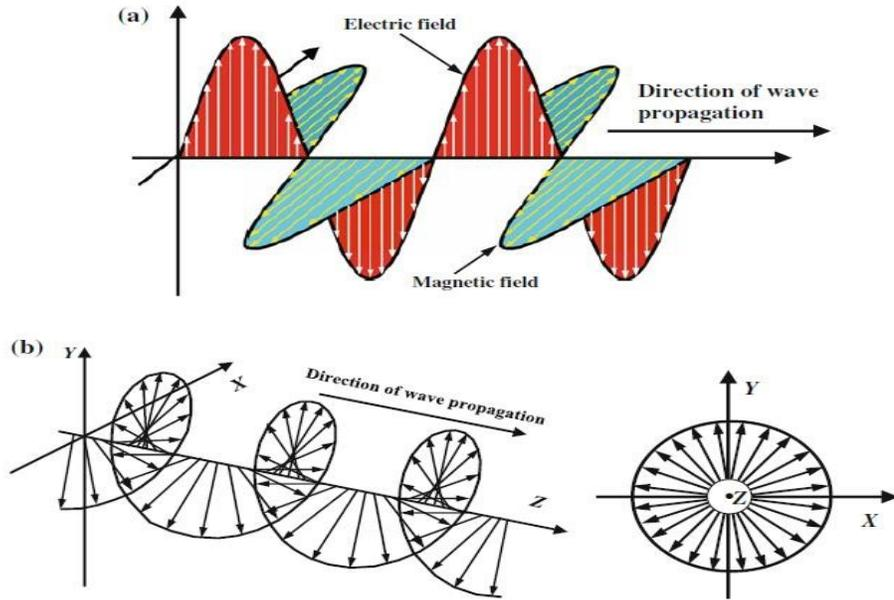
Figure 2. Electric field vector in (a) linearly and (b) circularly polarized beams
