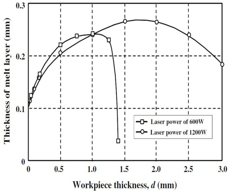
Figure 4. Effect of laser power and workpiece thickness on melt layer thickness
