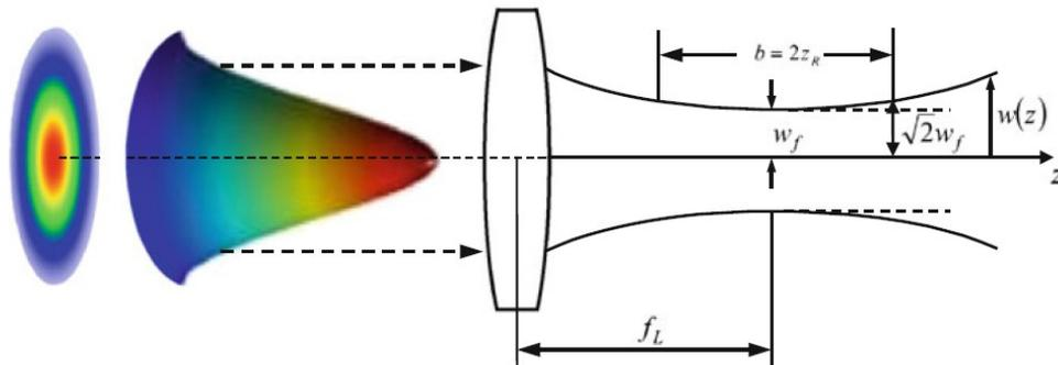
Figure 1. Distribution of power and focusing of TEM00 Gaussian-mode laser beam
