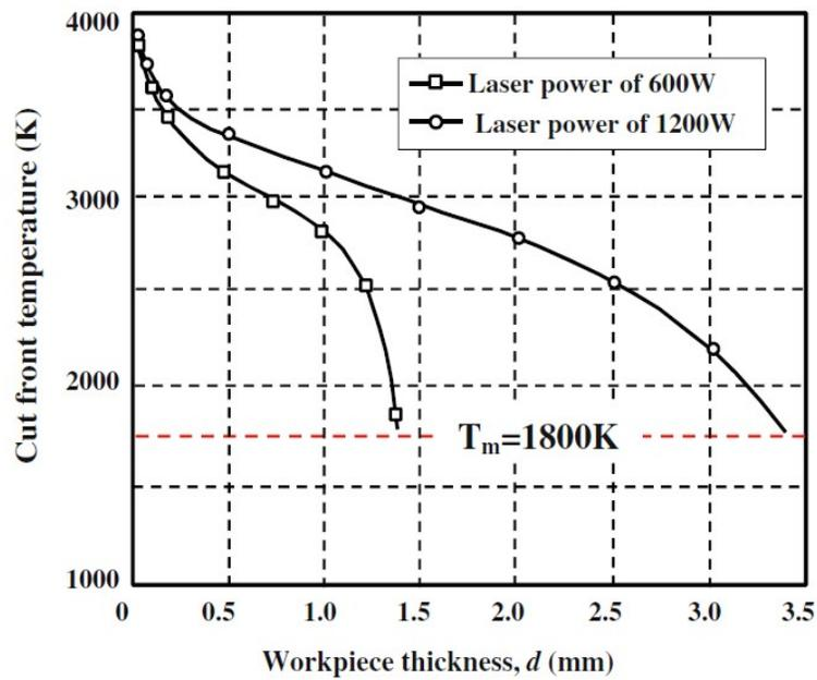
Figure 5. Effect of work piece thickness on the cut front temperature
