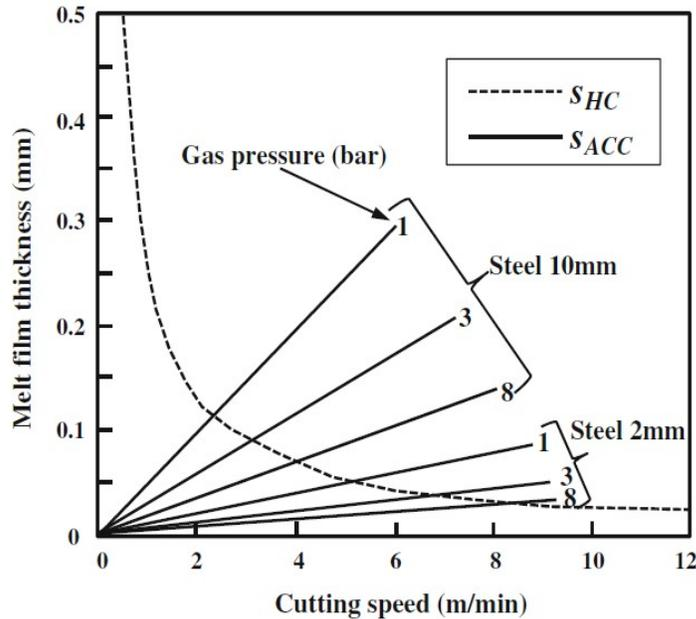
Figure 6. Melt film thicknesses of  $S_{HC}$  and  $S_{ACC}$  as function of cutting speed, gas pressure, and workpiece thickness
