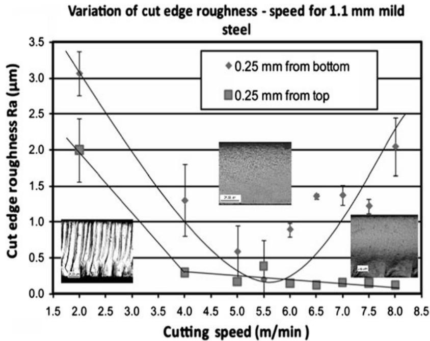
Figure 7. Variation of surface roughness at 0.25 mm from top and bottom surfaces with cutting speed during fiber laser cutting mild steel with oxygen jet
