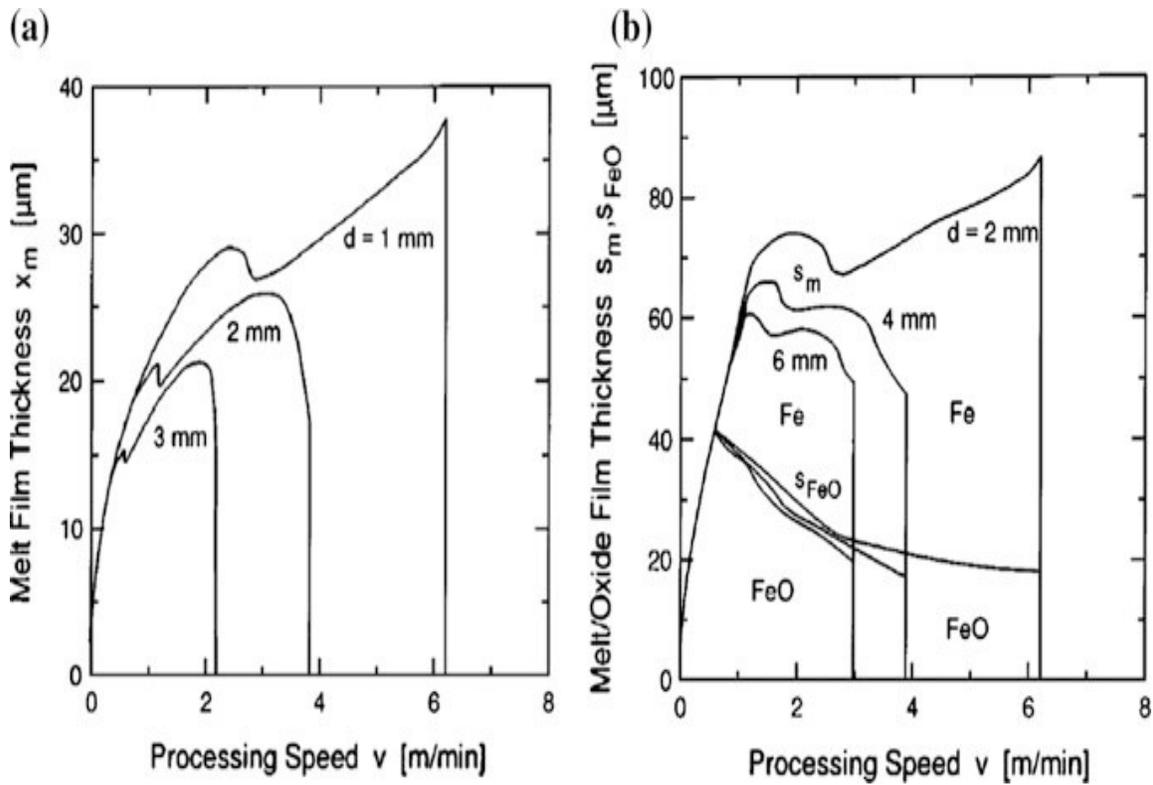
Figure 3. Melt film thickness as function of cutting speed and workpiece thickness in (a) laser fusion cutting and (b) reactive laser cutting
