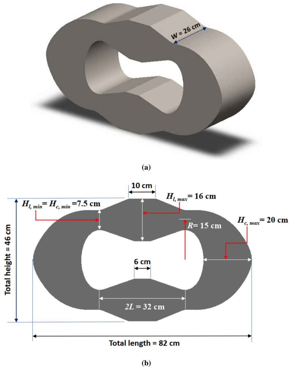
**Figure 6.** Optimum dimensions of the proving ring using (a) isometric view and (b) front view
