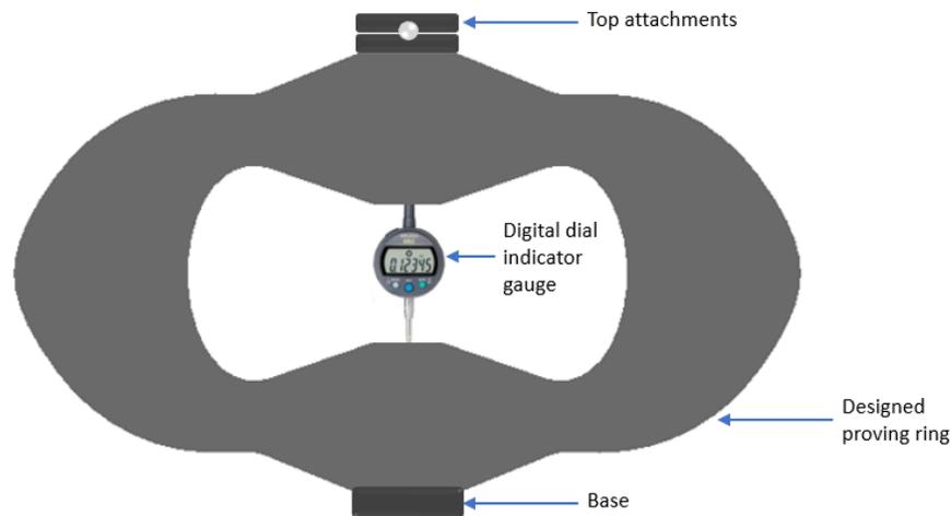
**Figure 10.** Illustration of complete proving ring structure with necessary accessories
