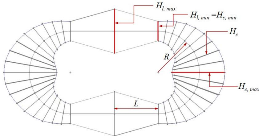
Figure 2. 2D front view of the basic structure of the proving ring for analytical design
