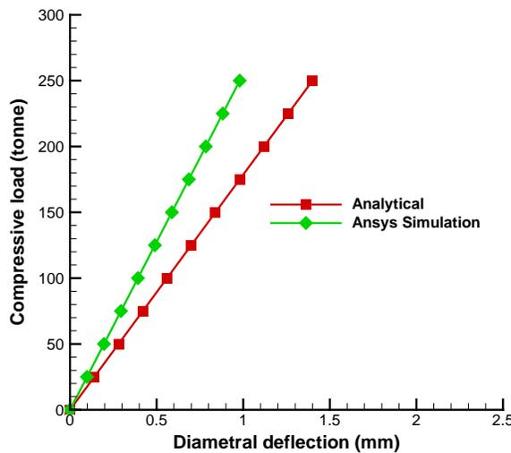
**Figure 9.** The variations of the diametral deflections of the designed proving ring for different applied loads
