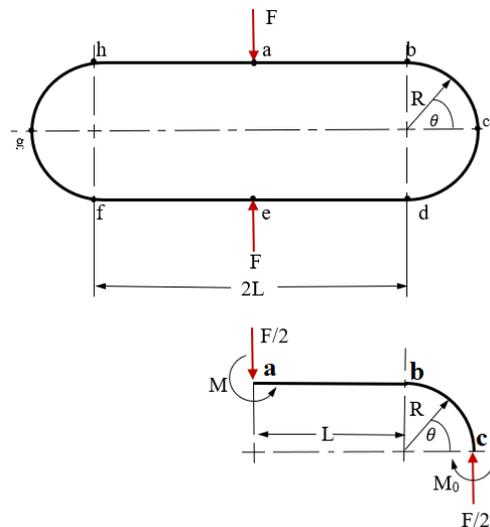
**Figure 1.** Free body diagram of diametrically loaded capsule shaped ring
