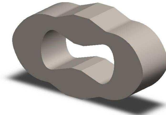
**Figure 4.** Isometric view of the developed 3D model of the actual capsule shaped proving ring
