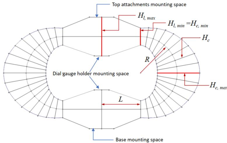
**Figure 3.** Modified 2D front view of the basic structure of the proving ring with necessary mounting spaces
