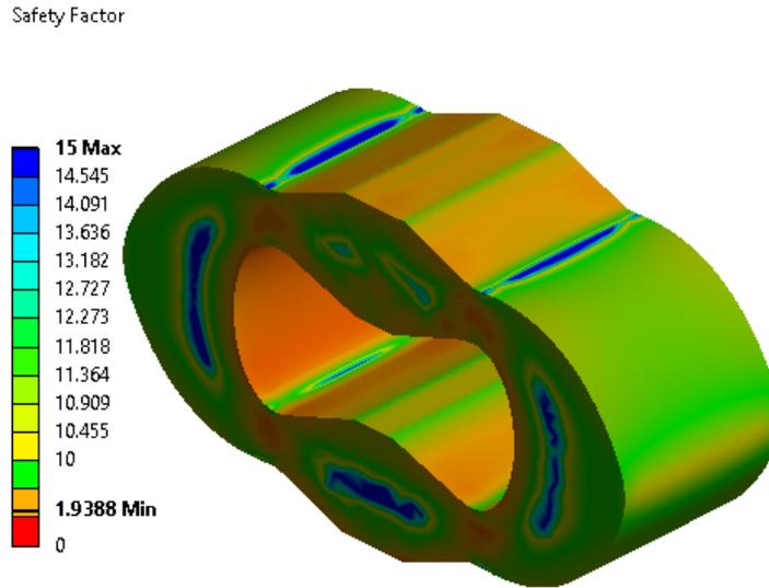
**Figure 8.** Numerical results for safety factor at different portions of the proving ring
