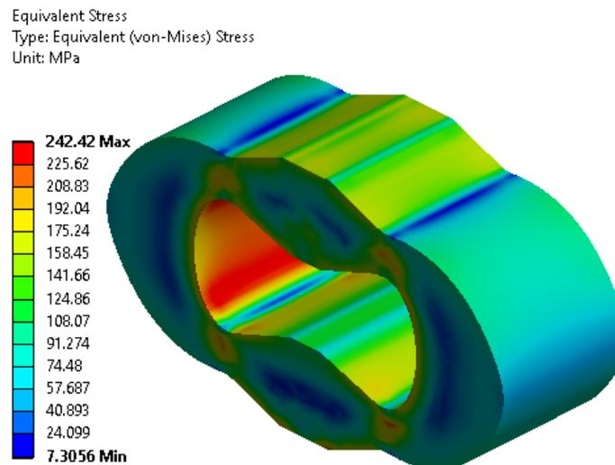
**Figure 7.** Numerical results for equivalent von Mises stress at different portions of the proving ring
