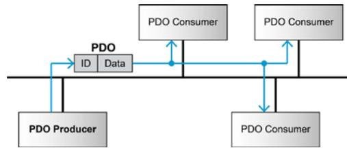
Figure 2. Process Data Object (PDO) [Adapted from Maxon motor ag "EPOS4 Positioning Controllers Communication Guide", Edition 2019-11, Doc ID: rel8759]
