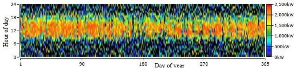
Figure 11: Inverter output in a year
