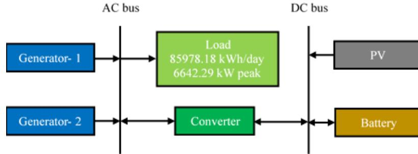
Figure 5: Diagram of the proposed hybrid power generation system
