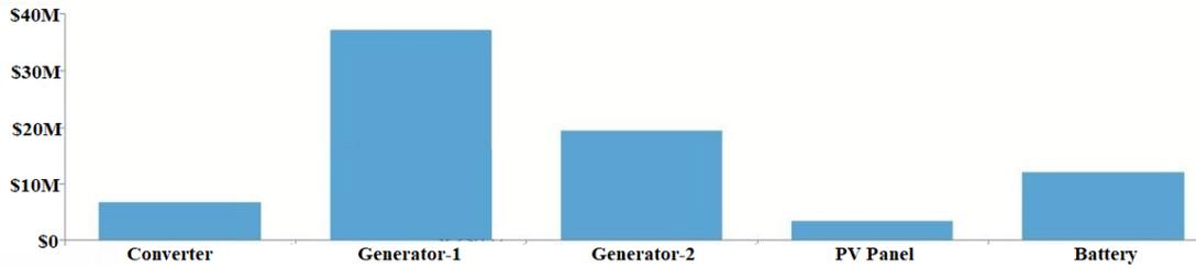
Figure 17: Net present cost by components
