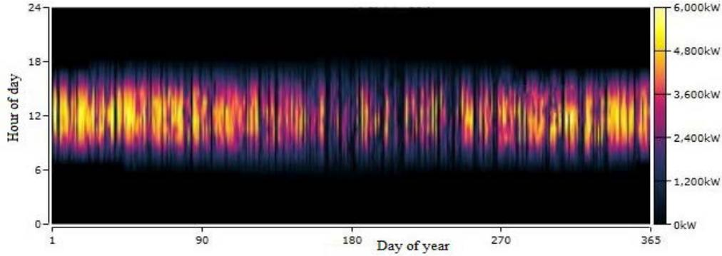
Figure 9: Annual power output by PV panels
