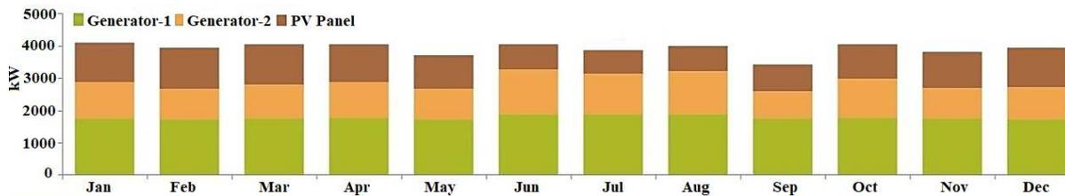
Figure 13: Monthly average electricity production by generators and PV panels
