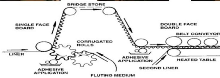
Fig 3: Production of corrugated fibreboard (courtesy of The Institute of Packaging)
