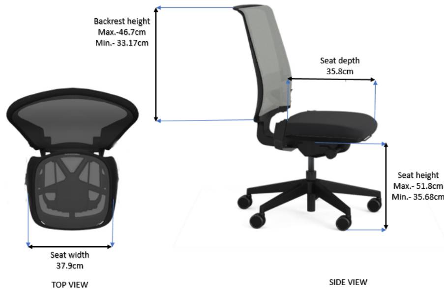
Figure 03: Proposed design of the adjustable chair
