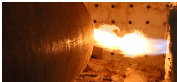
Figure 7: Heat treatment of pressure parts
