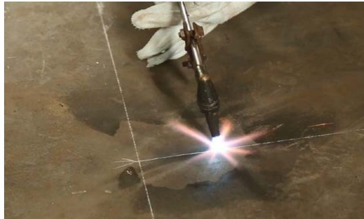
Figure 3: Cutting of metal sheet
