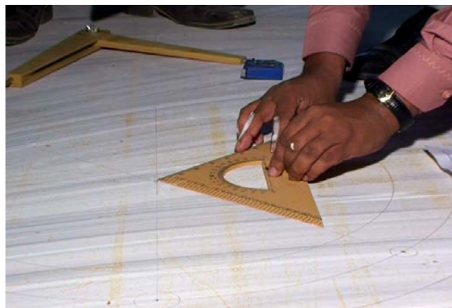
Figure 2: Marking metal sheet according to design
