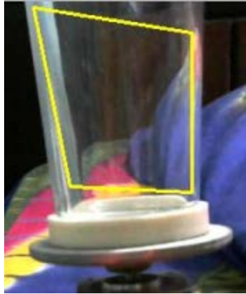
Figure 11: Captured Image in OpenCV, which can't detect any defect of glass bottle
