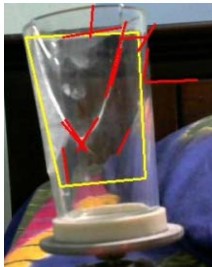
Figure 8: Captured Image in OpenCV, which detects the crack and bubble of glass bottle
