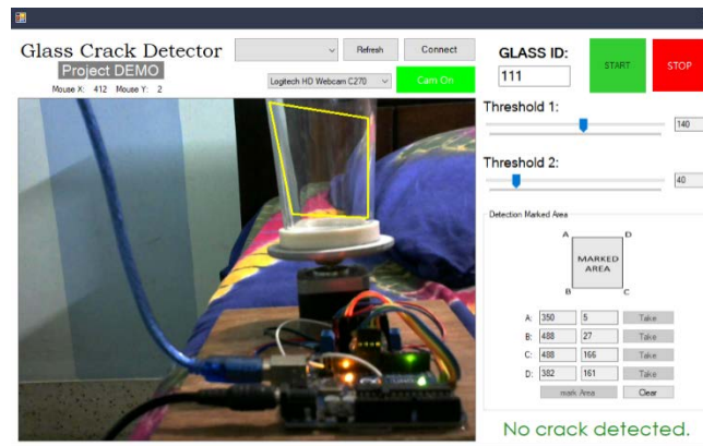
Figure 10: OpenCV detects no defects in glass bottle
