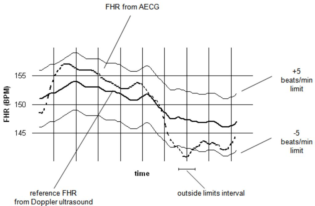
Figure 5: Comparison of FHR from ultrasound (solid line) and that of using signal processing system (dotted line) (each vertical division = 5 sec.)
