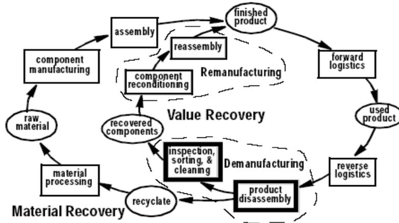
Figure 1: A typical manufacturing –remanufacturing system.
