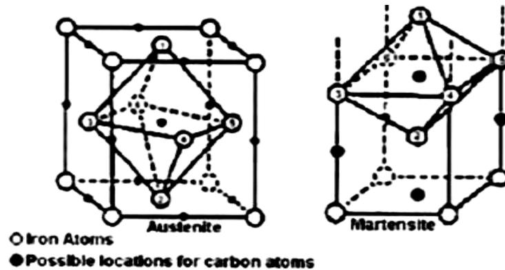
Figure 3: Atomic structure of Austenite crystal (left) and Martensite crystal (right) [2]
