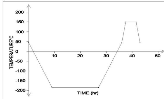
Figure 2: Time Vs Temperature for cryogenic cycle [2]
