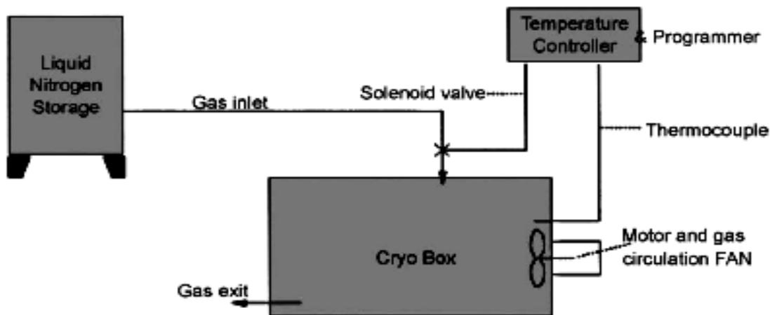
Figure 1: Schematic of cryogenic equipment [23]
