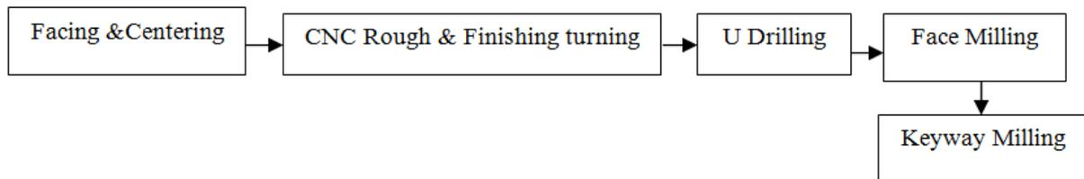
Figure 4: Machining process flow of crank shaft [2]
