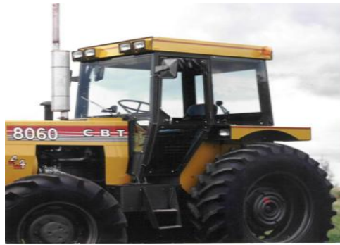
Figures 1. Bulky ROPS mounted on commercial farm tractor
