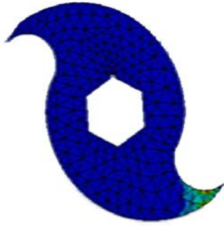
Figure 6. Stress on the blade by static structural method
