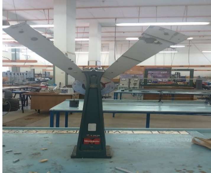
Figure 3. Charpy Impact testing equipment (UZ Mechanical Engineering Laboratory)
