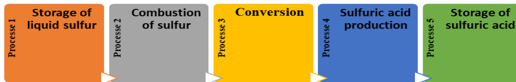
Figure 3. The 5 processes of the phosphoric sulfuric workshop
