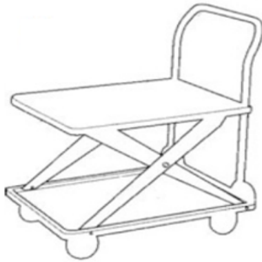
Figure 6: Mobile lifting Platform to lift and carry wooden logs
