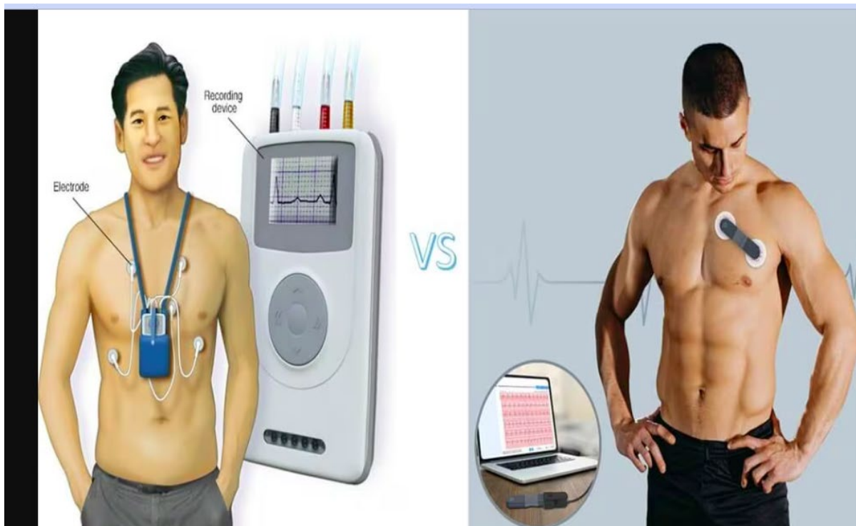
Figure 6. Side by side comparison of Holter ECG monitor (Left) and an IoT enabled wireless ECG sensing device (Right).
